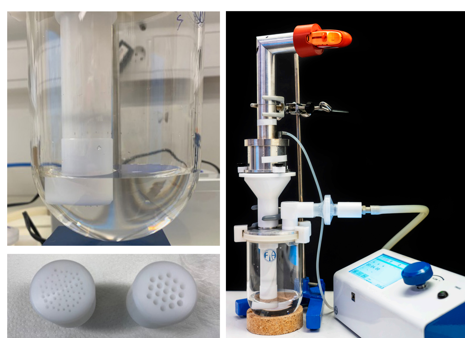
Figure 1. Photos of the Direct in Vessel aerosol collection apparatus.
